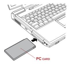
Figure 8-1 Installing the PC card
